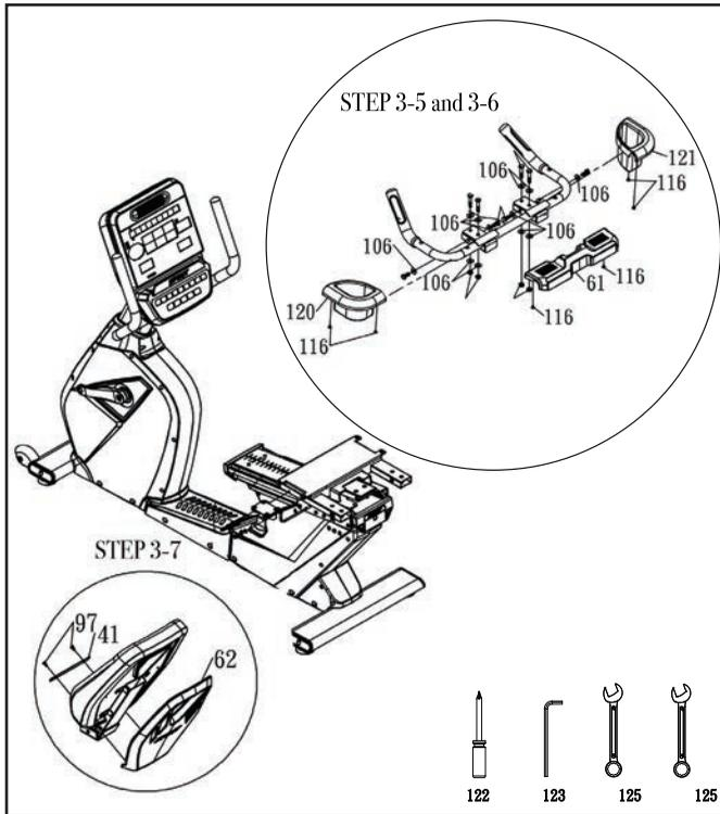
5. Attach REAR HANDLE BAR COVER (61) to REAR HANDLE BAR (6) using 2 SELF TAPPING SCREWS (116).
