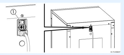
NOTE: When the power switch is set to the ON (I) position, the warmer automatically does a self-check and calibration of the iv bag detection system. Each warming position on the shelf illuminates blue, then green to indicate successful calibration.
