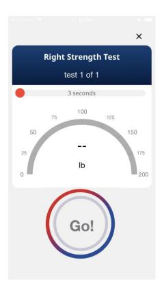
Once the test is started, force applied to the device will be displayed in the app.
