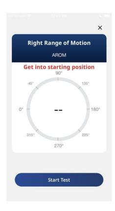
The Activforce 2 device is capable of measuring angles in any of the three axes, but only one angle, in a single plane of motion, should be measured for each test.
