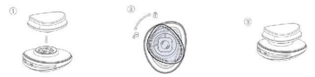
To release the attachment, twist the attachment counter-clockwise (toward the unlocked symbol) and lift the teeth out of the locking mechanism.
