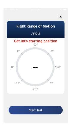
Place the device and/or subject into the starting position for test measurement and press the "Start Test" button. After calibration, move the device from the starting position (Position 1) to ending position (Position 2) through ONE plane of movement only (frontal, horizontal, or sagittal).
