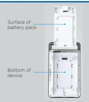
Insert the surface of battery pack on to the bottom of the device, make sure the bottom of battery is on the outside.
