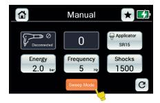
In this mode, you can set the modulation output for frequency and energy. The output of frequency and energy will conduct from minimum to maximum to minimum as cycles.
