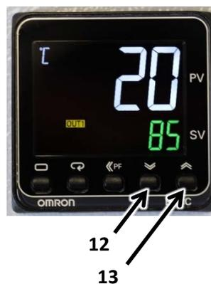
It is possible to set the target temperature digit by digit. See method below.
