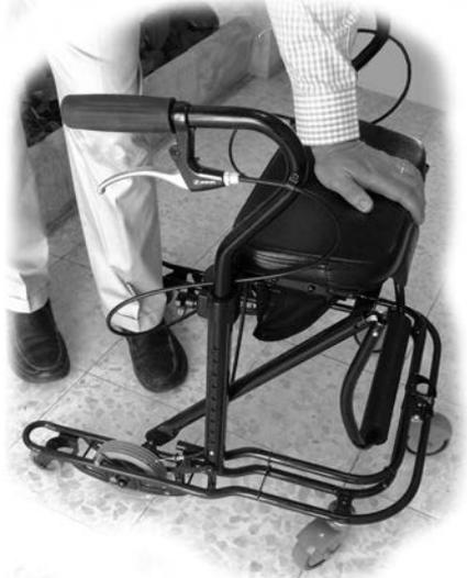
5) **Adjusting the Handlebars** to the proper height. Generally, the handlebars are adjusted so that the handles are 2-3 inches above your palm when your arm rests at your side.
