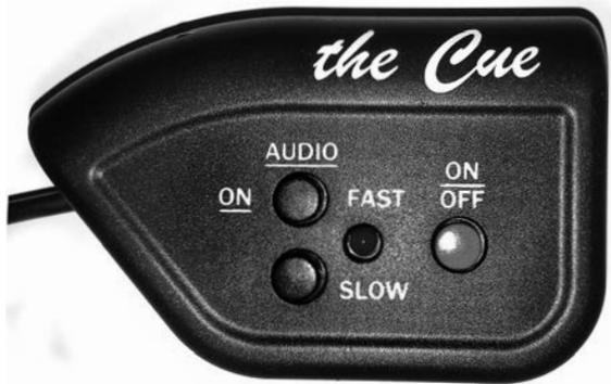
To activate Sound Cueing, press and hold the top black button in for a few seconds until you hear a steady clicking. In this mode, the two black buttons increase or decrease the cadence (speed) with each brief press. The cadence varies from 59 to 130 beats per minute over 15 increments.
