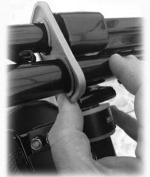
4) Pull up the handle bars until the seat becomes perpendicular to the ground. *(Below left)*
