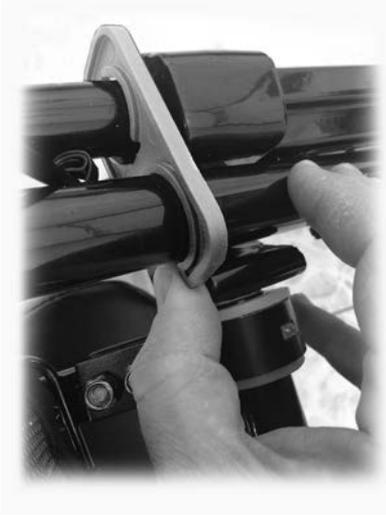
3) Secure the locking clip to stop the walker from folding. Simply rotate the clip until it attaches to the backrest tube.
