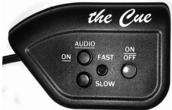
off period from 4 to 28 minutes in increments of 4 minutes; each click that sounds after pressing the button indicates 4 minutes of operating time in effect (from 1 to 7 clicks). Pressing the lower button lowers the click volume in steps to the softest setting, then recycling to the loudest setting.
